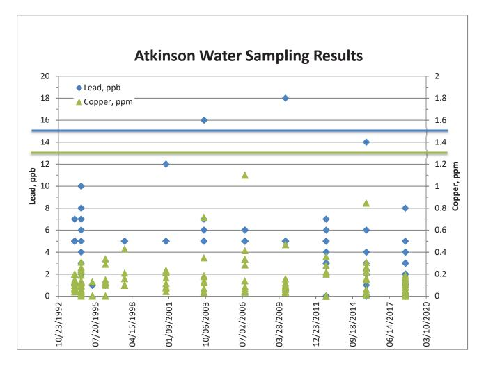
Figure 5 shows that recent sampling results for both lead and copper concentrations within the Atkinson area of the water system are below the regulatory action levels of 15 ppb and 1.3 ppm, respectively. However, Figure 5 shows historical lead levels have been above 15 ppb.
