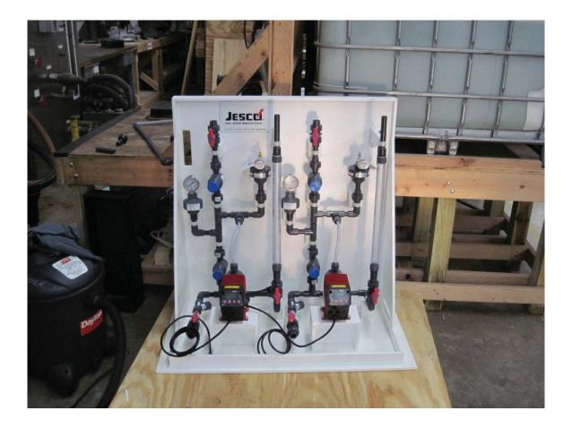
Although the existing chlorine feed pumps at the well sites may be sized appropriately to provide the necessary pumping capacity to feed chlorine for chloramine production, the above 2-pump package system could operate as two ammonia feed pumps (with one pump on standby).
